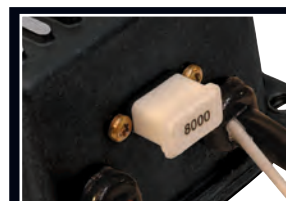
The 6 HVC-L Ignition features a built-in rev limiter.
